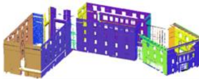
Figure 15. Image. RANSAC Model Imported to Revit
