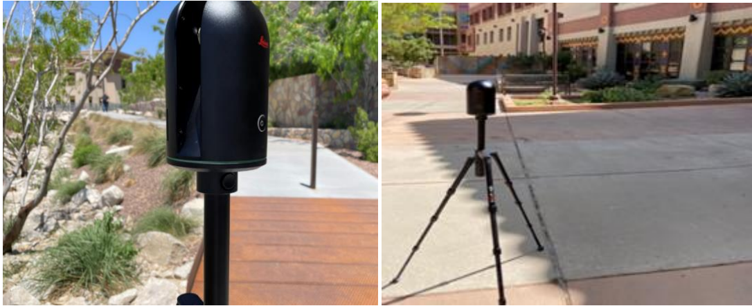
Figure 8. Image. Leica BLK 360 Terrestrial Laser Scanner (left) and sample set-up (right)
