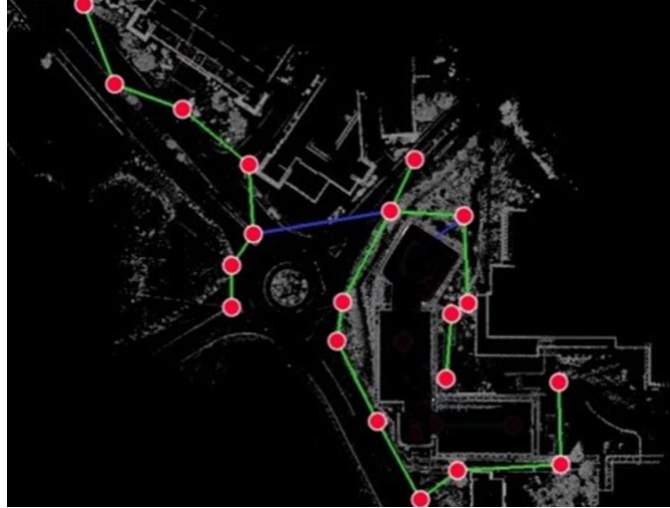
Figure 9. Image. Aerial-View of Scanner Location Placement
