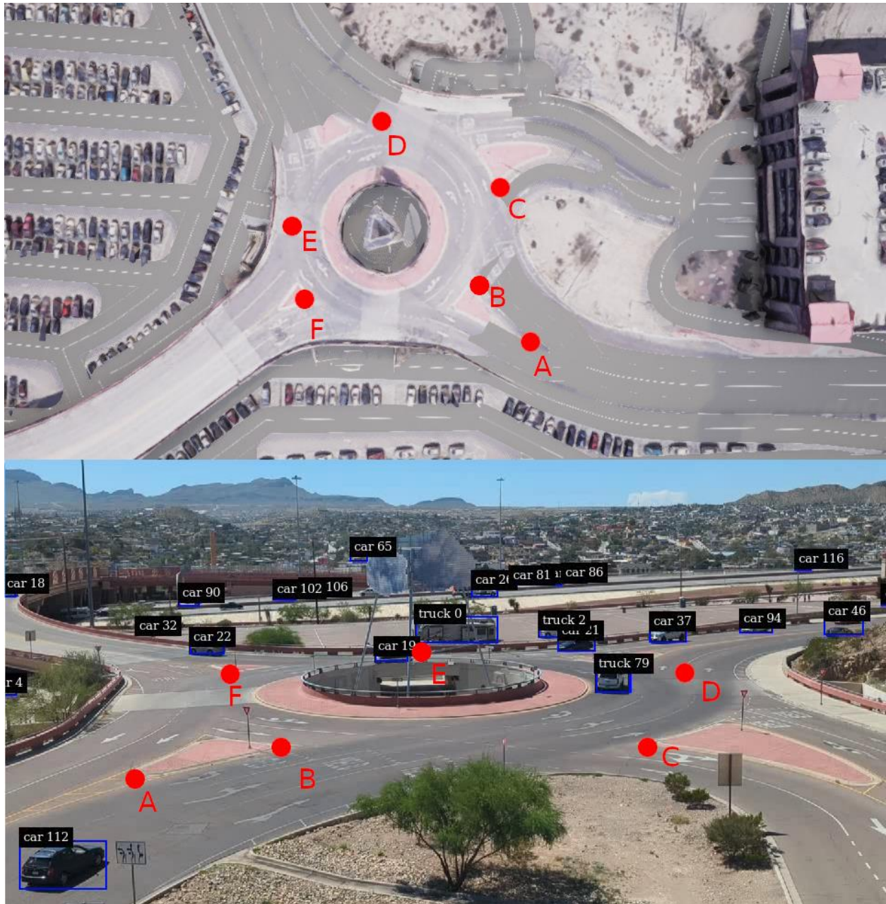
Figure 19. Points chosen to find linear transformation between two coordinate systems
