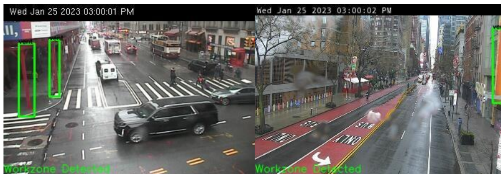
Figure 13. False positive example: Incorrect steam vent detection
