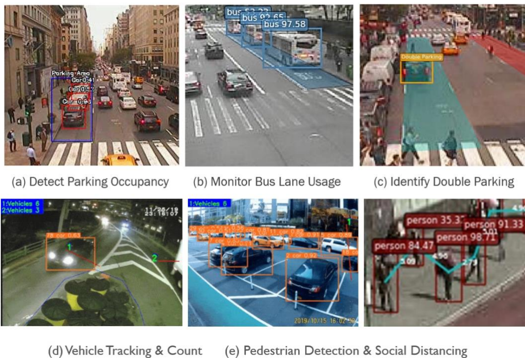
Figure 2. Computer Vision Applications Using Traffic Cameras (Source: C2SMART)
