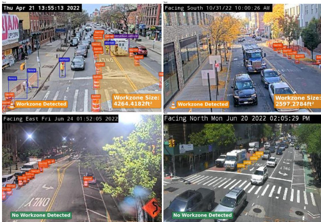
Figure 18. Output of work zone detection, inference, and area estimation.
