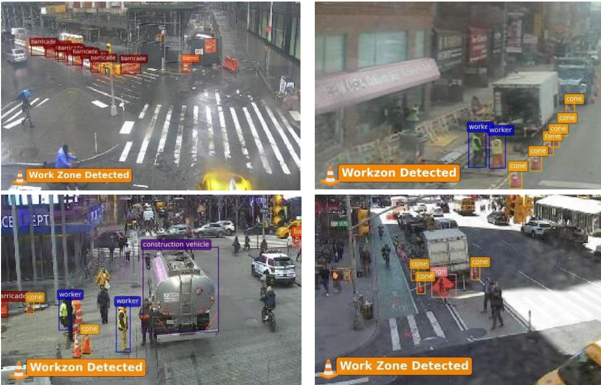
Figure 16. Example of detection output (daytime)
