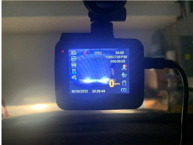
Figure 3-8 The Dash Camera used in the Data Collection System
