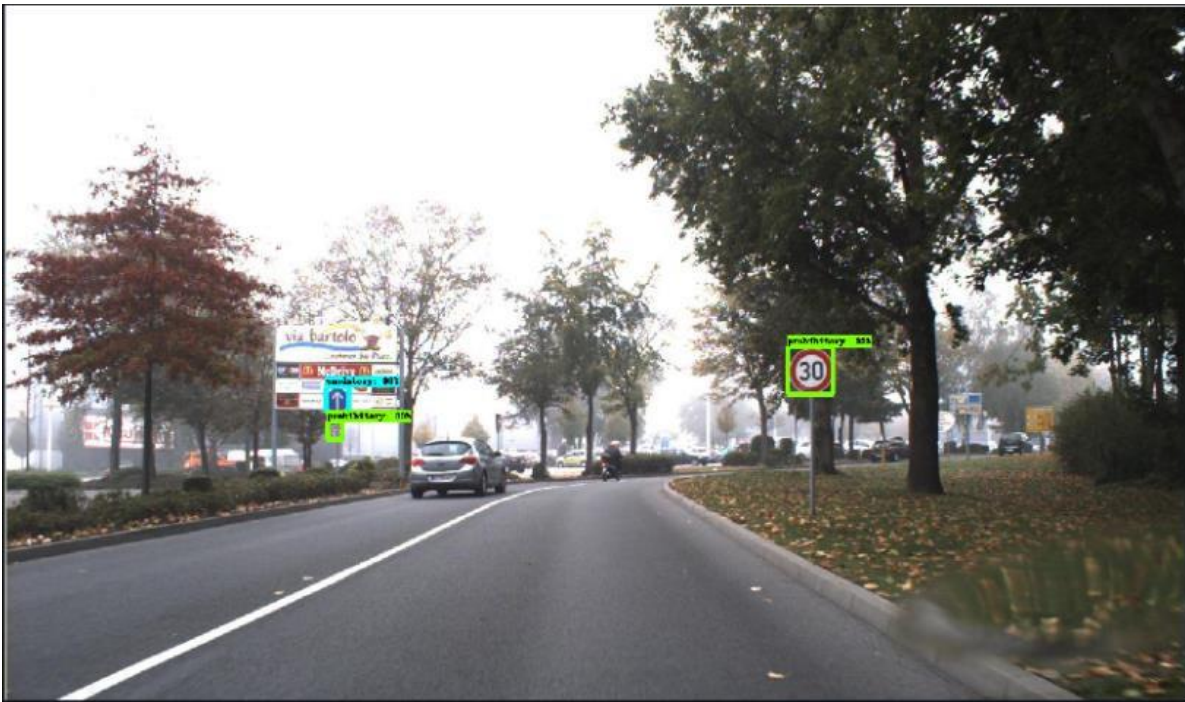
Figure 4-1 Sample Detection Results by Faster R-CNN Inception V2 based TSD Model Pretrained by GTSBR Dataset and Finetuned by Self-collected Data.
