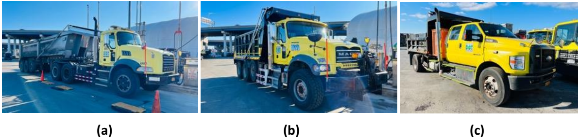
Figure 8: Calibration Trucks; (a) R1-Class 9 (886T), (b) R2-Class 6 (243FF), and (c) R3-Class 5 (106E)
