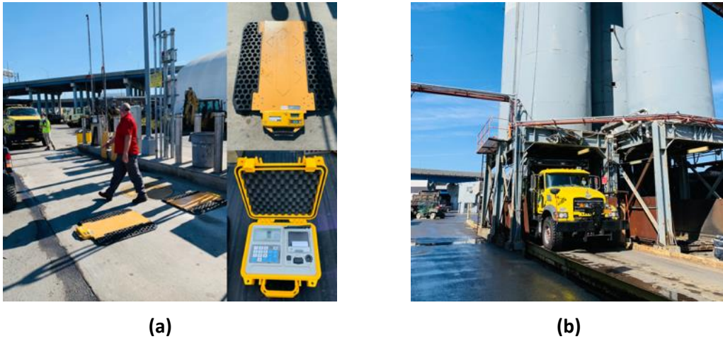
Figure 9: Weight Measurement using Portable Scale and Static Scale; (a) portable, and (b) static
