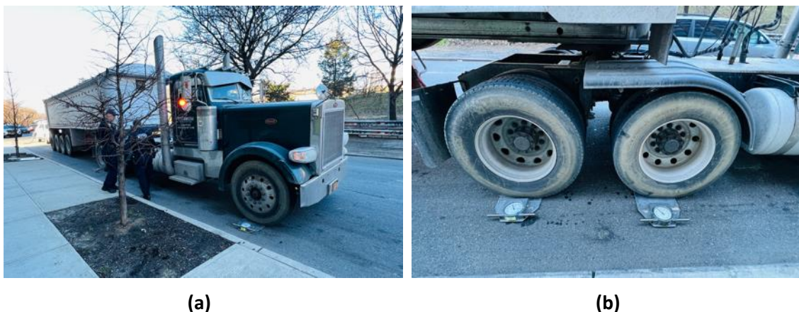
Figure 28: WIM Validation by NYPD; (a) NYPD Inspecting Truck and (b) NYPD measuring Axle Weights using Portable Scale
